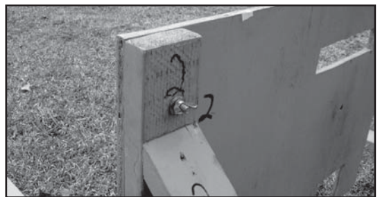
Barricade is secured to base legs with 1/4" bolts and wing-nuts. Barricade and legs are marked.
